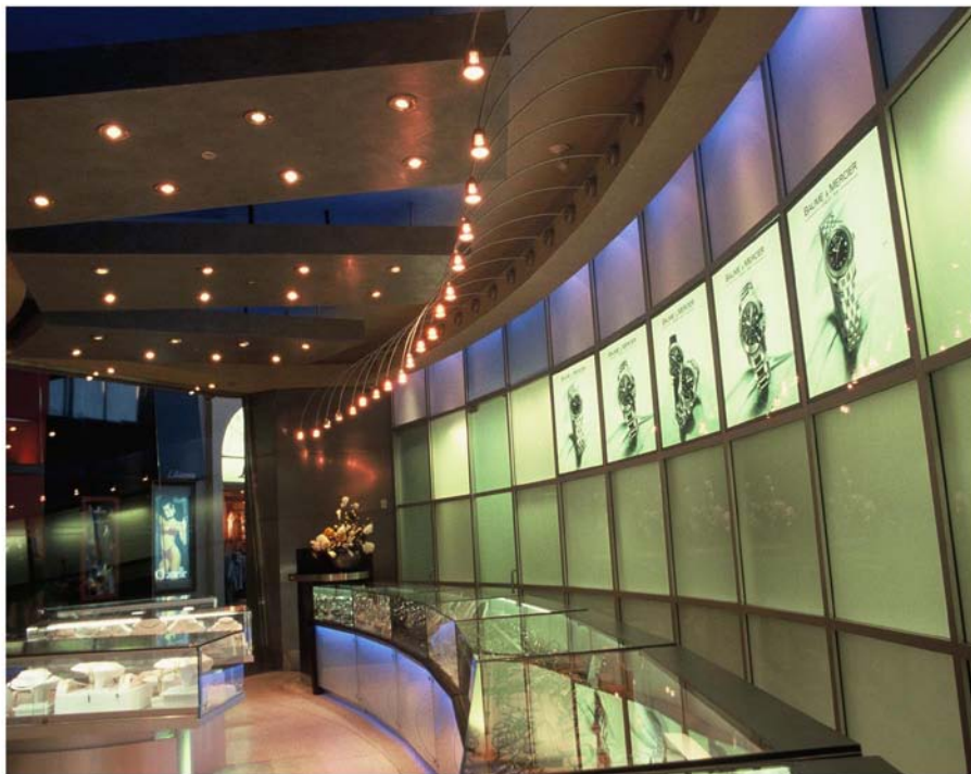
The curved back wall, which stands nearly 12 feet high and rises above the store's ceiling, is made of sandblasted glass illuminated from the rear. Above the wall, 24 lights extend outward on individual coils to light the showcases below.
